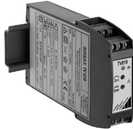
Fig. 1. Isolating amplifier SINEAX TV 819 in housing P12/17 , terminals not pluggable.
